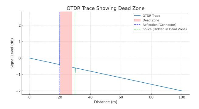
Here's a diagram of an **OTDR trace** showing the **dead zone**:
