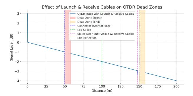
Here's the OTDR trace with **both launch and receive cables**:
