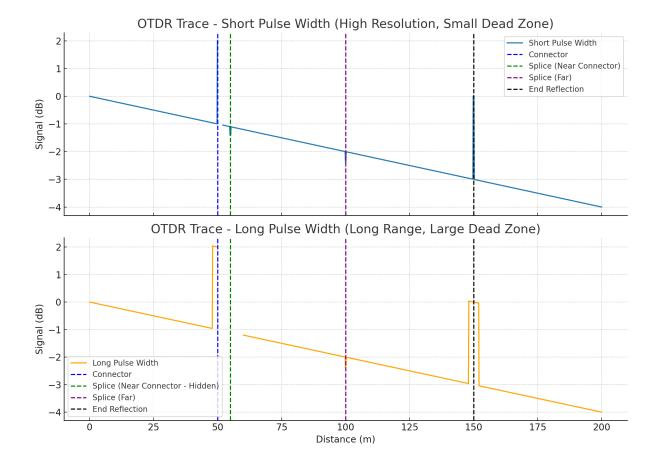
Here's the comparison between short pulse width and long pulse width OTDR traces:
